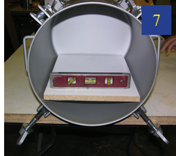
7 Place a board to use as a level surface inside the pressure chamber.
