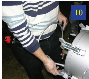
10 Use your body to hold the lid in place as you tighten the wing nuts.
