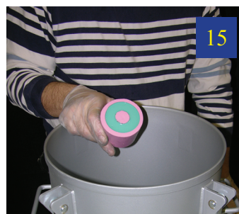
15 When the demold time is up, remove the mold from the pressure chamber.
