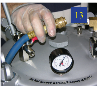
13 The air hose can then be removed and the chamber will retain its pressure.
