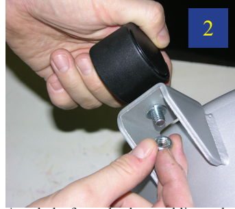
2 Attach the four wheel assemblies and secure tightly with a wrench.
