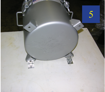
5 The pot is in working position and almost ready for pressure casting.
