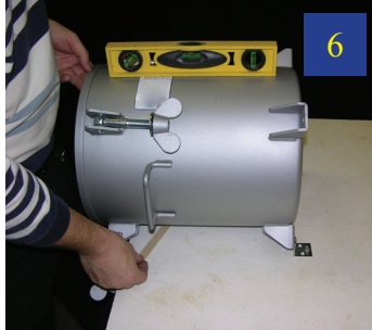
6 Make sure the chamber is level from front to back.
