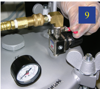
9 Flip the air control valve lever from the down position to the up position to release the air flow into the pressure chamber. Air will flow at 60 psi.
