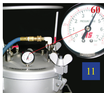
11 While the pressure pot's limit is 80 psi, it's not recommended to exceed 60 psi.
