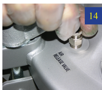
14 Keep the material under pressure for a duration at least equal to its demold time. Then release the air pressure valve.
