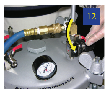
12 Close the air control valve by placing the valve in the down position.
