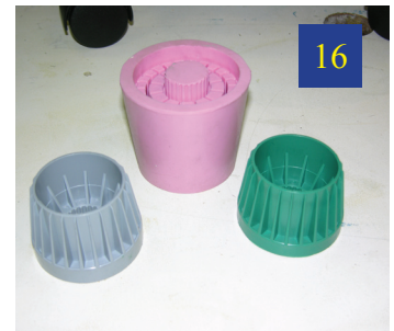
16 The result is a bubble-free casting that is identical to the original model.
